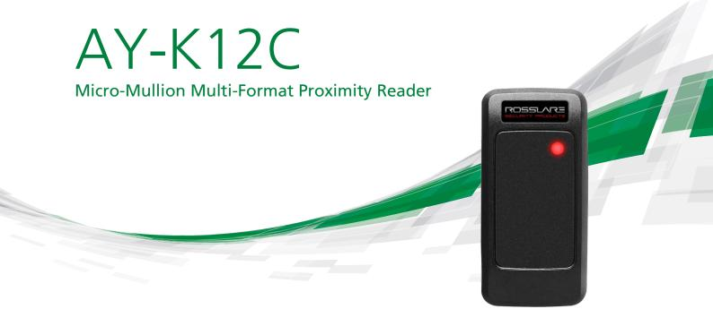
Rosslare's AY-K12C is a powerful RFID proximity card reader of 125-kHz cards and tags, featuring multi-format output and an excellent read range. The reader supports both standard EM and Rosslare format cards, and is highly flexible with behavior control options. With a sleek design and a tough UV-resistant and water-resistant casing, the AY-K12C is equally suited to indoor and outdoor use.
