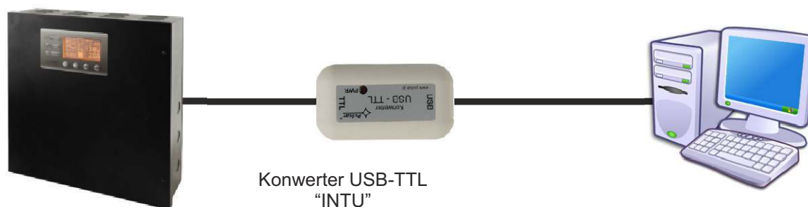
USB-TTL communication using the USB-TTL „INTU” interface.
